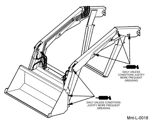
Lubricate all grease fittings: one at each end of lift boom arms and one at rod and base ends of each lift and bucket cylinders.
